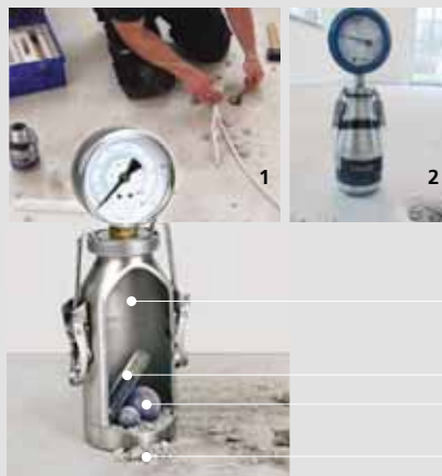
Gas acetylene Calcium carbide Stainless-steel balls for crushing Core sample
