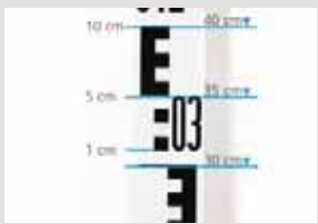
Long-distance scale with E graduation
