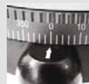
Freely rotatable horizontal circle
