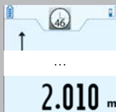
Timer function to automatically trigger measurement
