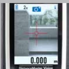
Viewfinder to target the measurement area
