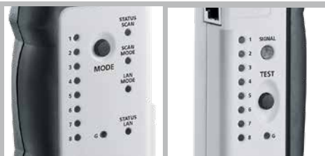
Assignment of individual conductors in LAN network cables
