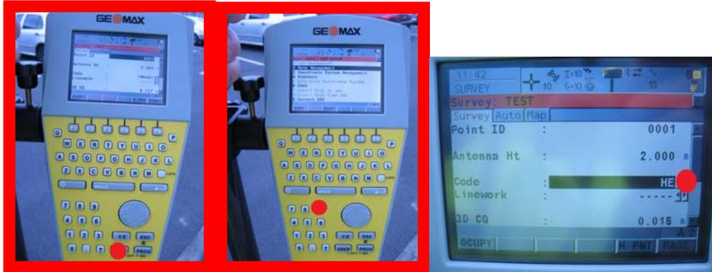
5. **Press USER on keyboard followed by 9 on keyboard (NB: Frequently forgotten).** At this stage on the top of the screen you should see a 'doppler wave' between the @ icon and the 'lightning strike' icon
