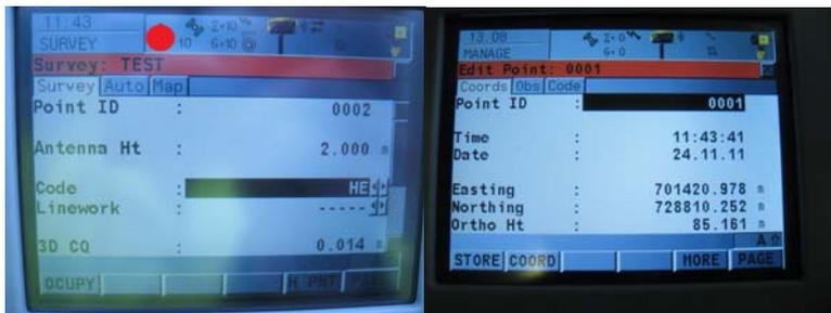
8. You can display the co-ordinates by clicking on the position cross on the top of the screen. Press CONT to continue surveying.
