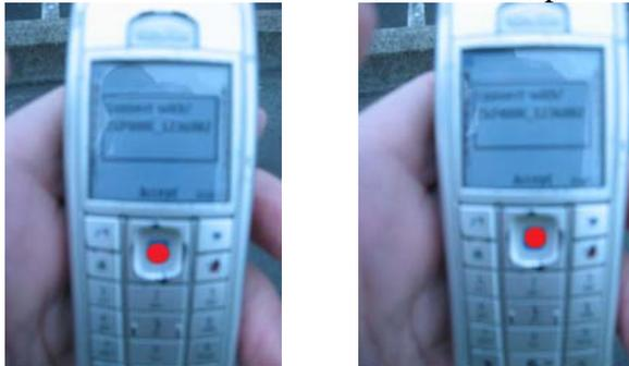
2. When phone displays "Connect with ZGP800 Accept?" – press centre button to accept. It will display a 2<sup>nd</sup> time and you should accept a 2<sup>nd</sup> time.
