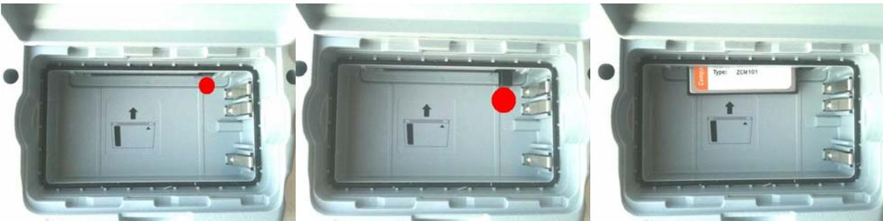
5. Remove the battery and press on the button in the top right of the compartment. When the button pops out press on it again, and the CF card will pop out.
