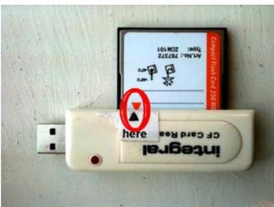
6. Align the arrow on the CF Card with the arrow on the card reader and push it gently into the card reader.
