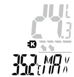
! The Min/Max values are deleted when switching modes and when the device is switched on/off.
