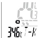
The device automatically switches to contact temperature mode T-K as soon as a temperature sensor (K-type) is connected. With a minimum battery charge of 15%, the device does not switch off automatically while the temperature sensor remains connected.
