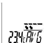
Max/Min/AVG modes refer to the infrared temperature and show the maximum, minimum or average infrared temperature. With the trigger (9) pressed, the Max/Min/AVG values are determined while measuring. The value is deleted and calculated again at the start of a new measurement or by pressing the trigger (9).
