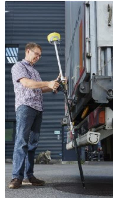
➔ In those cases it is mandatory either to switch off the Single mode at all and measure in conventional way, holding the pole vertical or if not possible, to use the dual mode to eliminate the magnetic influence.
