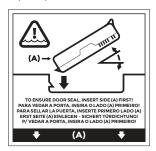
Hold the battery so that the black tab on the front edge of the battery is up and facing the door latch (this tab helps you pull the battery out). Place the back edge in first, gently pushing it underneath the two battery catches. Rotate the front edge down until it is in position.
