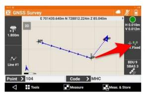
Tap on RTK Fixed to access the GNSS Status screen
