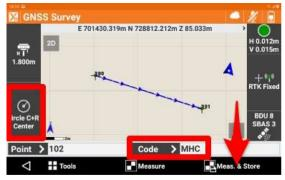
Double tap on the screen to open the CAD drawing
