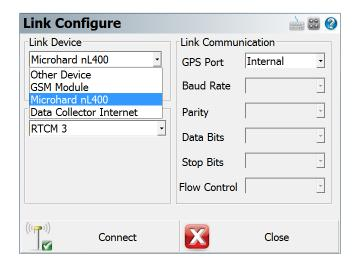
Set the Data Format with the required RTK base message type. When selecting **GSM Module** or **Data Collector Internet**, tap Setup to define the NTRIP parameters. Once an internet connection is established, a suitable mountpoint can be selected.
