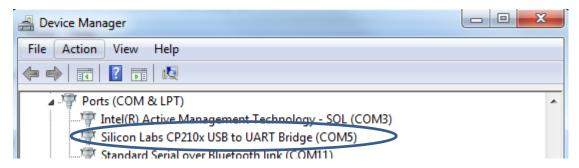
With the receiver connected to the PC, launch Assistant by clicking the respective icon in your Windows desktop. From the menu bar, select **File...Connect** and choose the COM port number as defined in Device Manager. The COM Port defaults are Baudrate 115`200, 8 databits, 1 Stopbit, Parity None.
