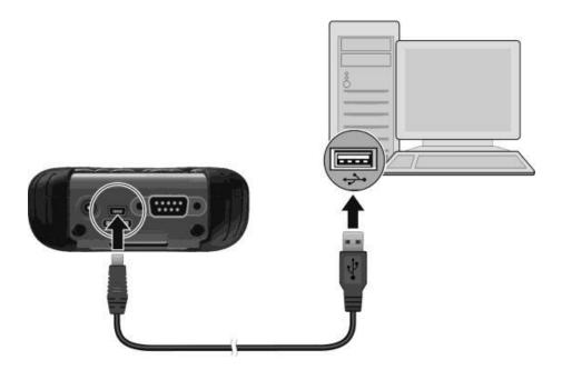
The device drivers will now automatically be installed. If the Windows **Found New Hardware Wizard** starts, click the Close button. After the drivers are installed, the Mobile Device Centre or ActiveSync will automatically start. The contents of the PS236 internal memory can be seen with Windows Explorer and are defined as a drive named **Portable Device**.
