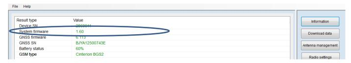
If the firmware is older as the one downloaded from the GeoMax download Area it is recommended to perform an update. To update the receiver firmware, download the
