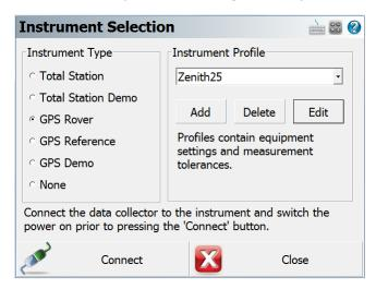
To ensure that measured heights are computed correctly, it is important to define the receiver type. At the *Antenna Height* panel, choose the Model as **Zenith15/25**. The Measured Height is the default length of the telescopic pole.
