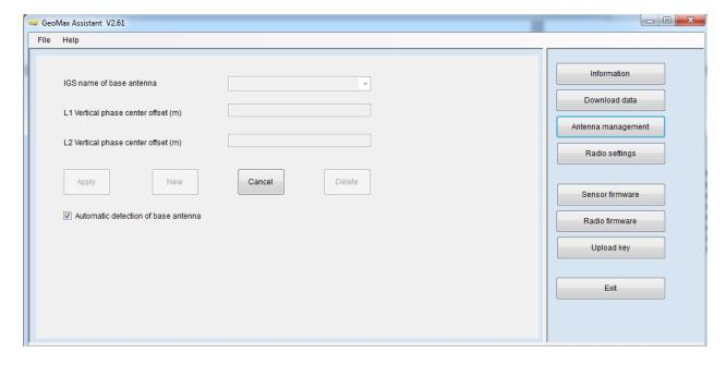
In order to add new antennas disable the function of the automatic detection of the base antenna by removing the check mark. Then click **New.** Enter the IGS name of the base antenna and the vertical phase center offset for L1 and L2 in meters (m). In order to add the currently missing GeoMax Zenith35 / Zenith35 Pro, please enter the following parameters.
