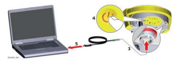
Download the USB cable driver installer CP210xVCPInstaller\_x86.exe from GeoMax Downloads. For 64-bit versions of Windows use the installer named CP210xVCPInstaller\_x64.exe. Run this file to install the USB port to Serial converter software by following the instructions of the Windows installer wizard.
