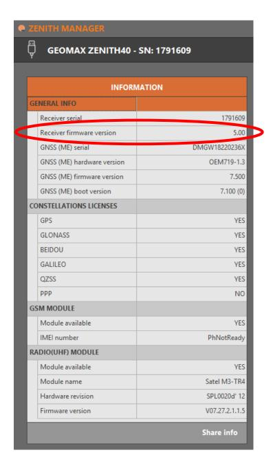
If the firmware is older as the one downloaded from the GeoMax partner Area, it is recommended to perform an update. To update the receiver firmware, download the respective \*.FW file, copy to the SYSTEM directory on a MicroSD card and insert it into the Zenith16/40 receiver. Select **Firmware Upload** from the bottom menu. The contents of the SYSTEM directory are displayed. Choose the required file and click **Upload** to install the firmware onto the receiver.
