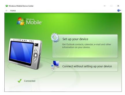
Locate the USB cable in the yellow container. Insert a fully charged battery into the GNSS receiver and switch it on. Connect the cable to the Lemo port of the receiver. When connecting the cable to a USB port of the PC, the cable's drivers will be initialized automatically and the aforementioned WMDC will appear showing that the receiver is connected.
