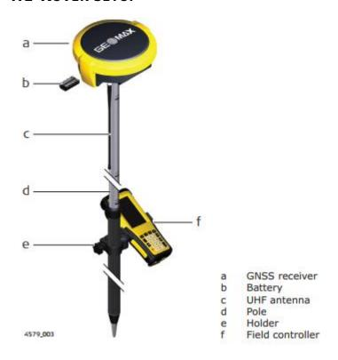
For a RTK rover, the Zenith16/40 equipment can be setup on a pole as shown above.
