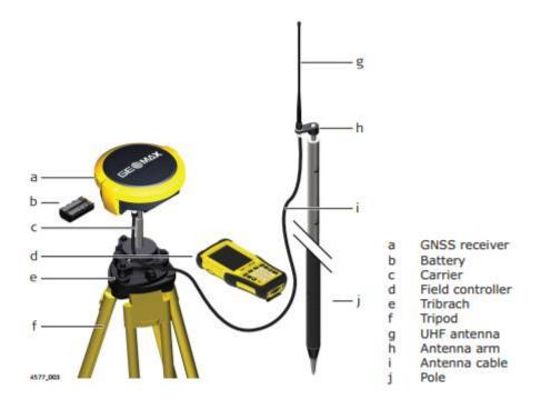
Attach the UHF radio antenna to the 760275 ZAR200 antenna arm. The arm has a 5/8" thread for mounting onto a telescopic pole or a tripod setup with threaded carrier. The antenna is connected to the Zenith16/40 using the 760266 ZDC202 cable. The required RTK output message can be configured using Zenith Manager or by field software.
