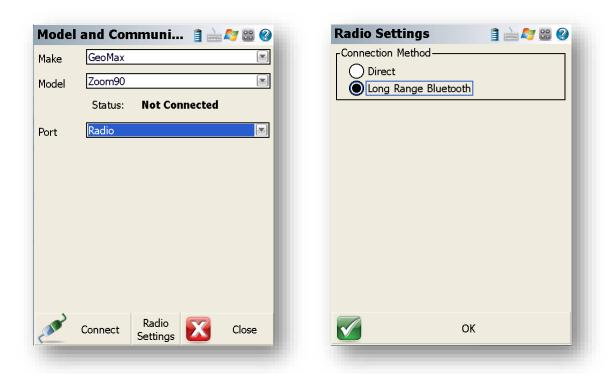
When everything has been configured correctly, tap *Connect*. The map view will then be shown and you are ready to measure. For further information on using Field Genius/Layout Pro for total station measurements, refer to the Field Genius/Layout Pro instruction manual.
