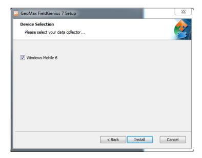
When prompted by the handheld for where to install, choose **Device**. Once the installation process is completed, the Field Genius/Layout Pro software can be started by selecting it from the Windows Start Menu.
